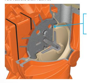
Elimination of outer piston abrasion and potential leak point for longer diaphragm life, especially when pumping dangerous and abrasive fluids.
